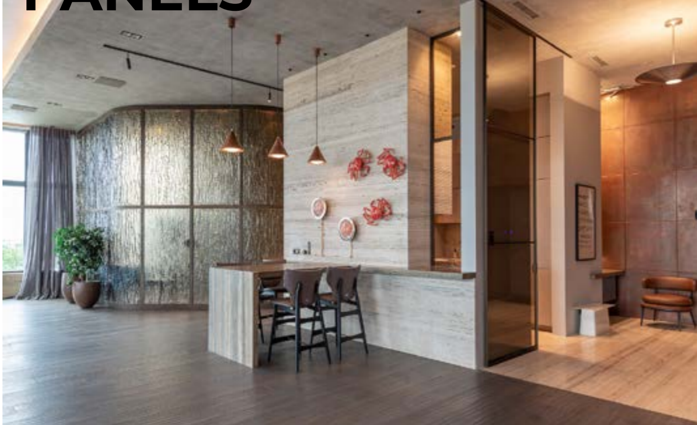
Interior zoning in a private interior Fresh.Glass texture: Bark (Oak) Materials: Glass, steel Technique: Kiln glass casting
